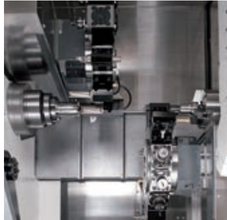
Upper-L, Lower-R boring operation
